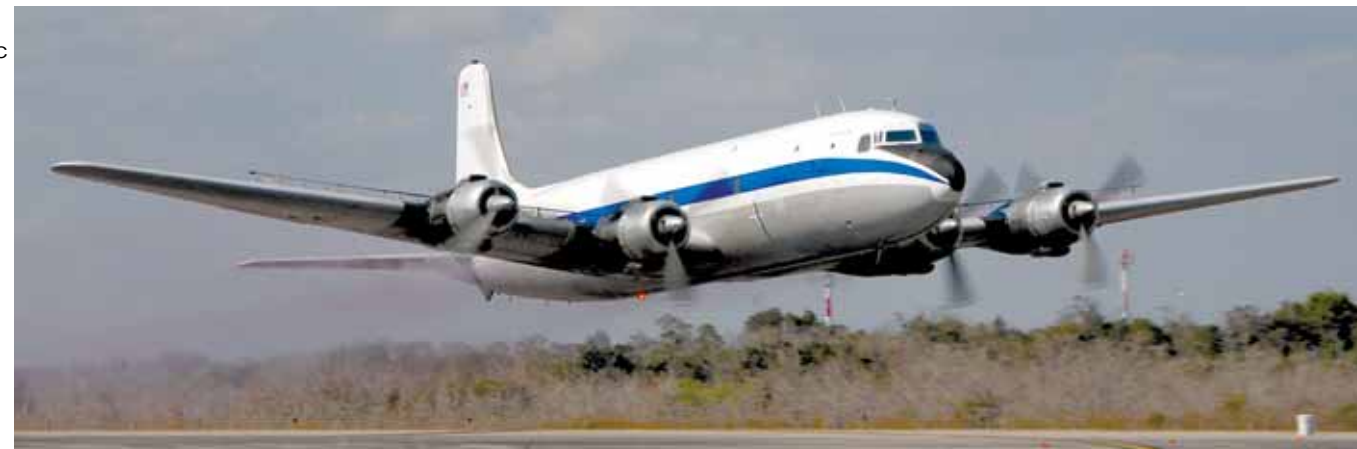
N70BF coming in for a low pass over sensor equipment on the runway at Dade-Collier Training and Transition Airport during the initial testing of the big Doug's spray dispersant system. This deserted airport is 35-mi west of Miami in the Everglades and was a perfect location for the testing.
