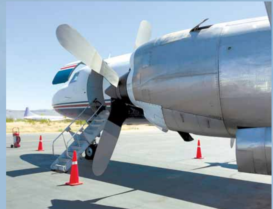
Allison 501-022G turbines of 4300-hp each power the CV5800 — almost double the power of the R-2800 piston engines installed in the original CV240/340/440 series. The stretched fuselage of the CV5800 gives the design a more elegant appearance. Note the ex-Linea Aerea Mexicana de Cargo CV440 XA-TDL parked in the background. (Paul Snyder)
