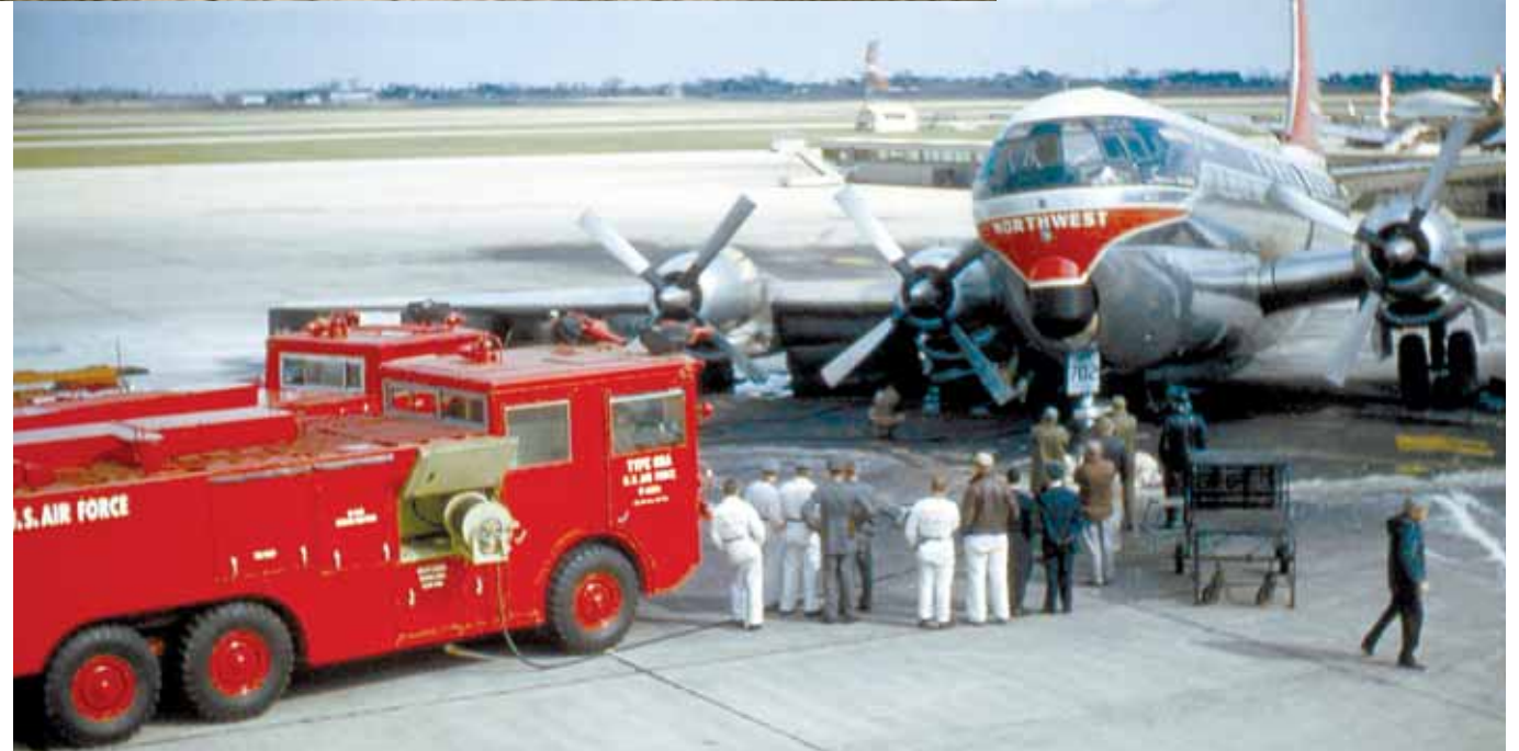
An Air Force crash crew took care of any fuel leaks after N74602's gear collapse. Number four propeller and R-4360 suffered damage. The aircraft made its first flight on 28 March 1949 and was delivered to Northwest on 22 June 1949.
