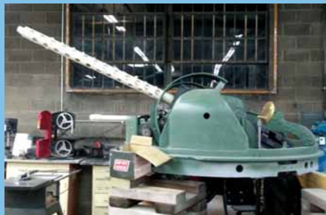
The Martin 250 turret provided by Carl Scholl of Aero Trader is seen under construction.
