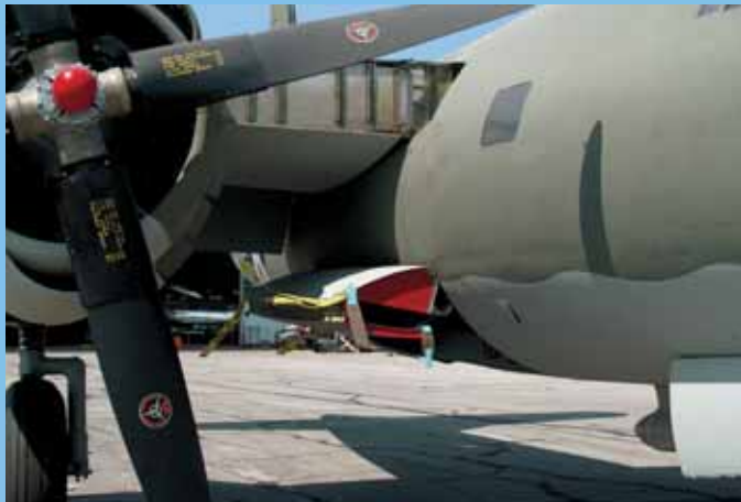
Bomb bay doors in place and open. Note the missing leading edge.
